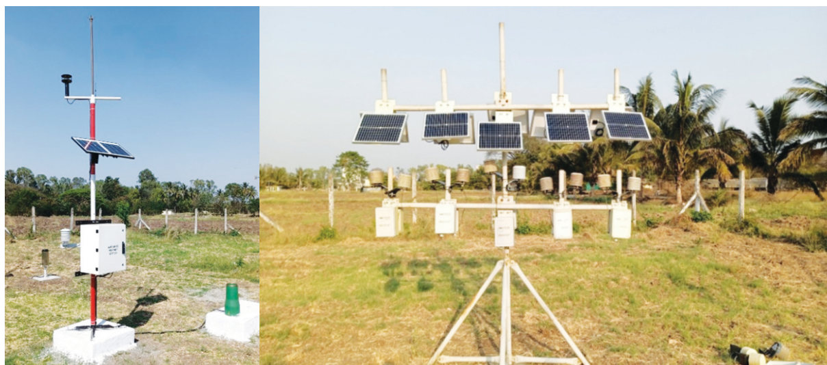
Figure 8: Sensors collocated with Reference Grade AWS for field calibration and comparison on field
